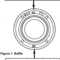
Air cap number located on face of cap - cap number must correspond with baffle number to assure 10 PSI cap pressure.
